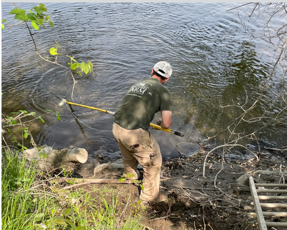
Harrison Bardwell of Bardwell Farm collecting an irrigation water sample for E. coli testing. Photo L. McKeag
