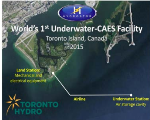
Figure 5.4 Illustration of Hydrostor’s UW-CAES demonstration facility in Toronto, Canada [Hydrostor, 2013]
