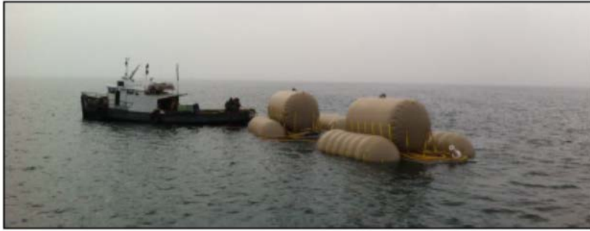
Figure 5.7 Barge transporting rigid storage vessels for Hydrostor’s Toronto project [Wanwalleghem, 2014]
