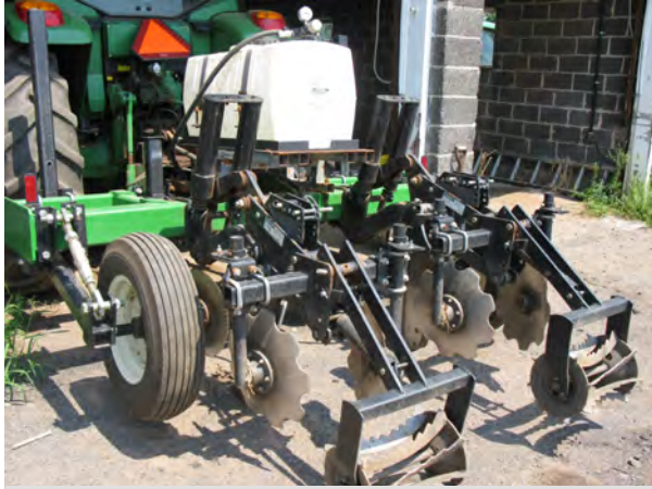
Photo- DZT machine with tank for placing liquid N below seeding depth at planting.
