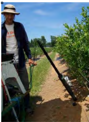
Figure 2. [left] Minirhizotron camera used to photograph roots of a blueberry plant in the field at the OSU North Willamette Research & Extension Center. [right] An image of blueberry roots taken with the minirhizotron camera. Roots are highlighted (red line = first-order root; green line = second-order root) using computer software designed to measure root characteristics. Photo credit: Luis Valenzuela, Oregon State University.
