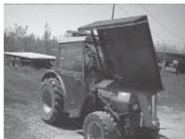
Figure 6. Flamer raised for easy transport and repairs or adjustments.
