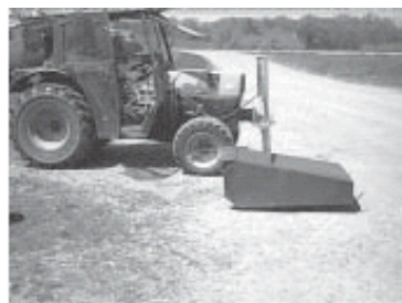
Figure 3. Flamer mounted on front of tractor.
