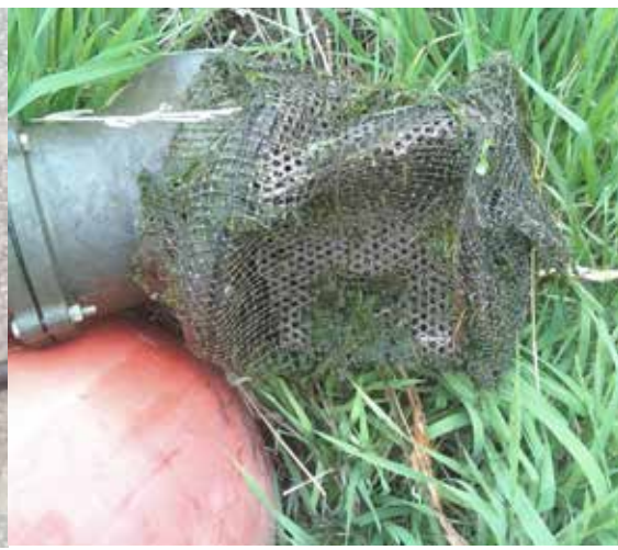
Too much suction destroys a clogged filter. photo: T. Hardy
