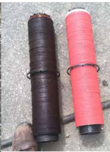
Disc filters after cleaning. photo: T. Hardy
