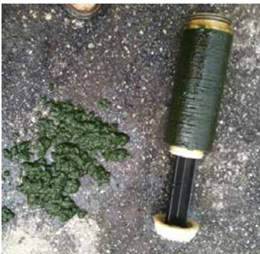
Algae accumulation on disc filter photo: T. Hardy
