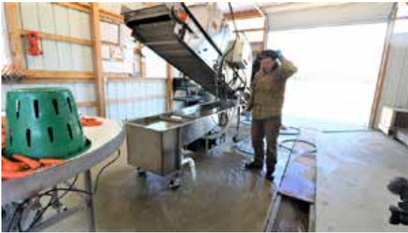
Hinged and lifted via pneumatic cylinders to make cleaning access easy! Photo: A. Chamberlin
