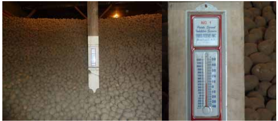
A thermometer to monitor air temperature in middle of potato storage pile (left) and close up of thermometer (right).
