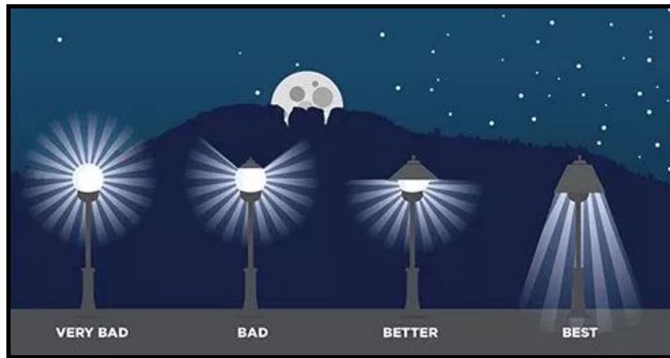
Figure 4.22: An illustration depicting what types of streetlights create the most light pollution. 46
