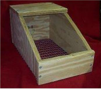
You need the following tools: an electric rotary saw, a screwdriver or drill (recommended) with both screwdriver bit and regular bit just smaller than the screws you will use, a hammer, and pliers. A table saw is handy for making some of the cuts, but is not necessary. You will also need 120 screws (we used #10, 1-3/4", but other sizes will work), fence staples, and 1/2" x 1" (or 1/2" x 1/2") metal wire mesh. You may need some sandpaper if you have rough edges.
