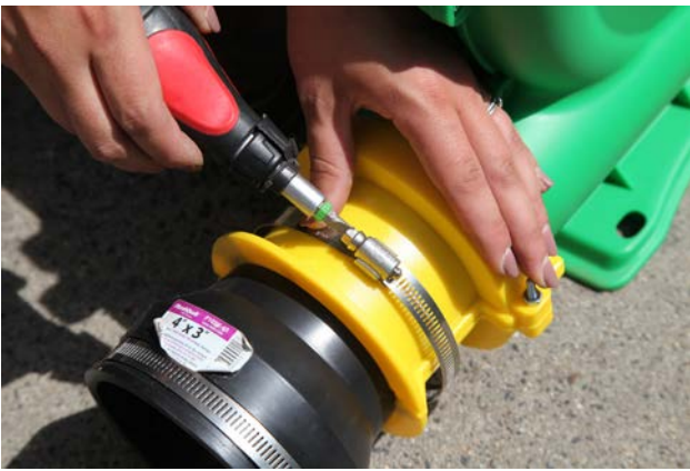
Figure 3. For extra hold use cast iron clamp to secure blower to coupling.
