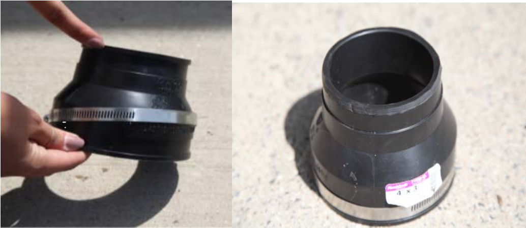
Figure 10. Cut off the lip of the 3" section of coupling.
