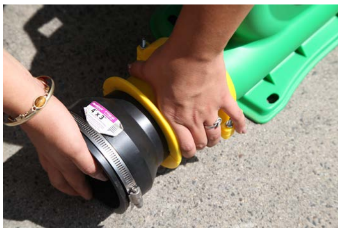
Figure 2. Connect pipe to blower with coupling and 1ft. pipe
