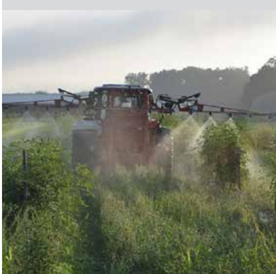
To spray this organic tomato variety trial, Katie drove the Rears RMCO, with a hydraulic fold boom and an auxiliary tank, 1 mph with a nozzle pressure of 60psi to put out 20 gal of water to 0.25A. In the tank was 2 quarts Cueva, 5 oz. Serenade Optimum and 2 oz. NuFilm for protection against late blight already found elsewhere on the farm. Photo, H. Godoy
