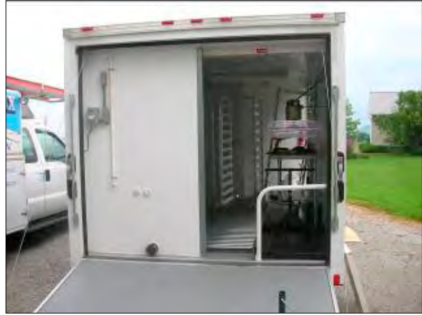
Back door of quick freeze unit - note ramp for easy access.
