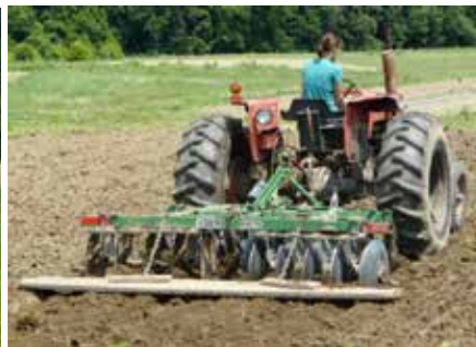
2) Immediately incorporate the residue with a chisel plow, rototiller, or heavy disc (photo).
