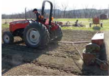
2) Using a Brillion Sure Stand (photo) or a Stanhay seeder at 12-15 lbs/acre can be effective if the soil is moist, but in a dry year, the brillion will simply push piles of soil over the seed, burying it too deeply.
