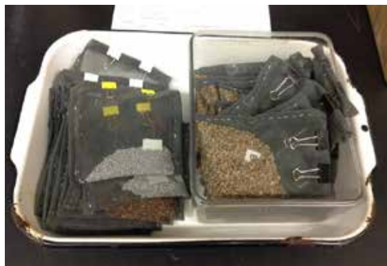
We use a strip of insect netting, folded in half and stapled along either side to make reusable treatment packets. The open edge of the packet is clamped shut with binder clips.
