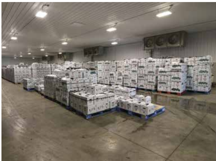
Keeping product off the floor and away from walls reduces the chance of freezing.
