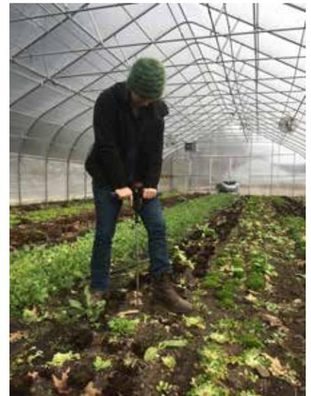
*Test soil compaction with a penetrometer.*
