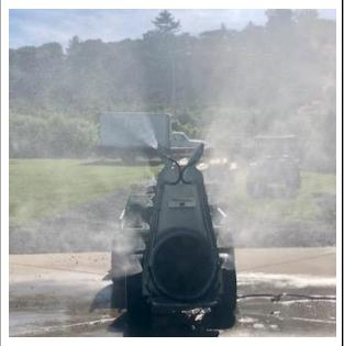
My, or actually OESCO's, little **Carrarospray airblast sprayer** outfitted with the tower accessory has a pretty good spray pattern I think. Six nozzles on each side, top four are air-induction, bottom two are hollow cone. Calibrated to deliver 50 gallons per acre at tall-spindle spacing. 50 gallon tank so I can spray an acre, reaches 10 to 12 feet high. Just applied some NAA at 2 ounces per acre for return bloom, along with Sysstem-Cal (Agro-K) at 2 quarts per acre.
