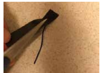
Cutting the electrical tape for increment markings
