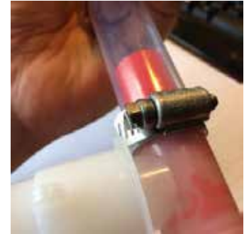
Tubing secured with hose clamp
