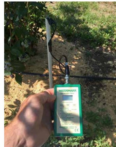
A handheld reader provides instant data useful for irrigation management decisions. Photo J. DeLisle
