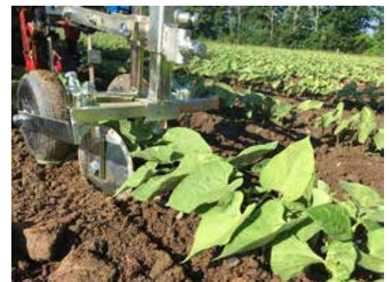
Figure 3. A small disk hiller with guide wheels.
