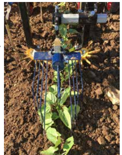
Figure 2. A row harrow (foreground) and finger weeders (background).
