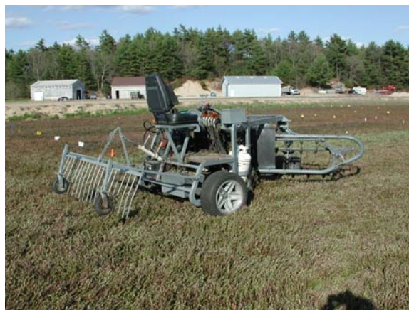
Grower-manufactured pruner with knives attached to a rotating head in front combined with a hydraulic rake attachment in the rear.
