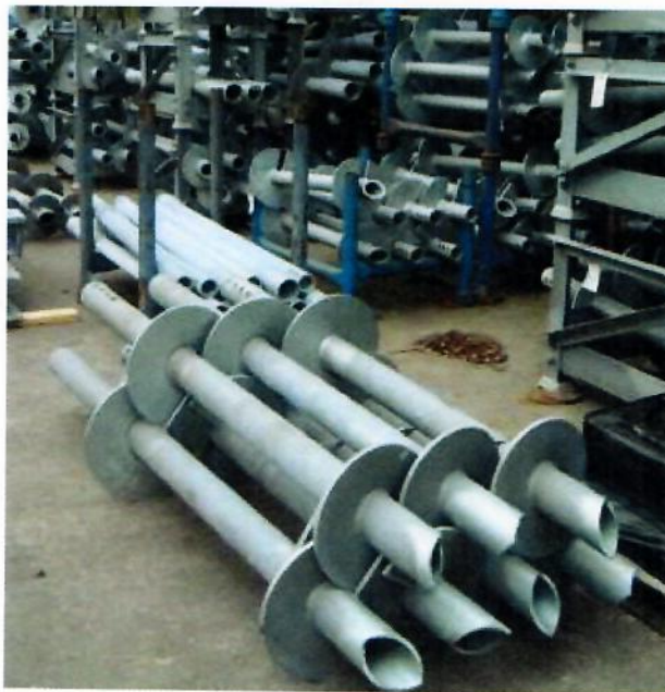
Figure 66. Helical Piles Consisting of Steel Central Shaft and Two Helical Plates.
