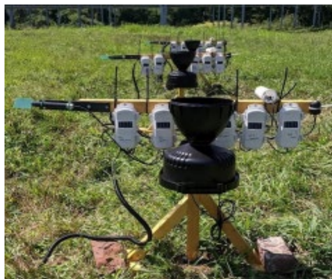
Figure 2. Mounting unit assembly with sensors.
