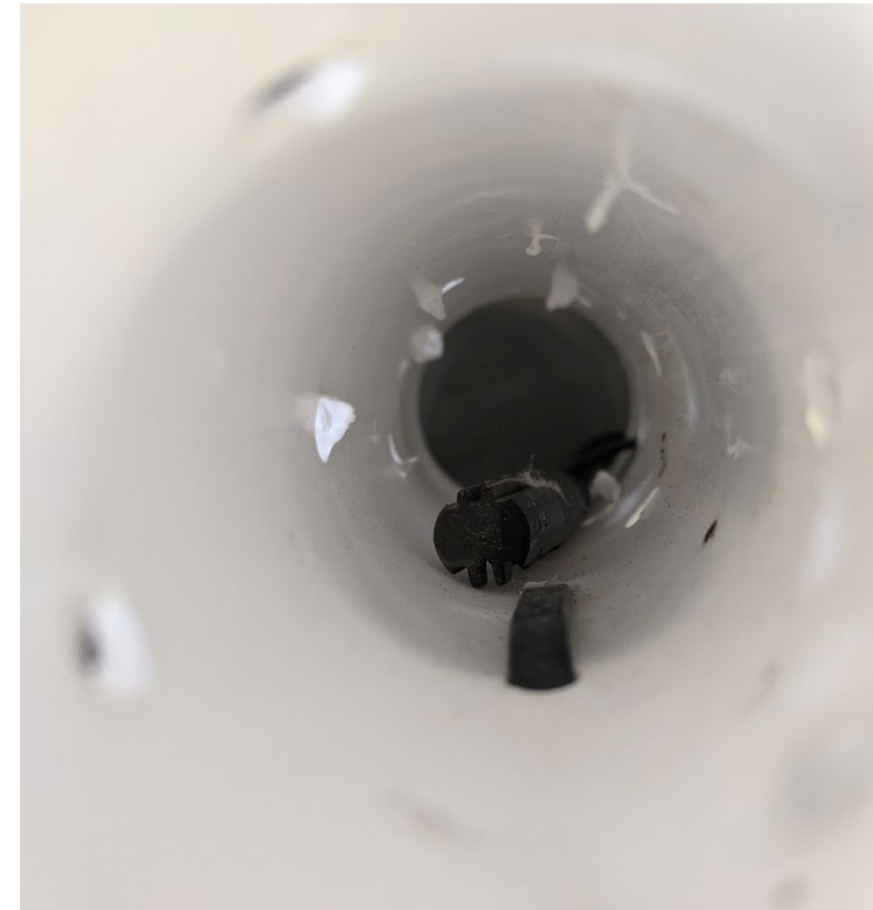
Figure 6. Interior view of PVC tailpiece. The sensor is placed inside the tailpiece and the wire is secured with a cable tie using a drilled hole. The whole tailpiece is connected to the stand through two drilled holes in the center. In 2023, a small block of wood will be glued to the interior of the tailpiece to elevate the sensor and improve airflow.
