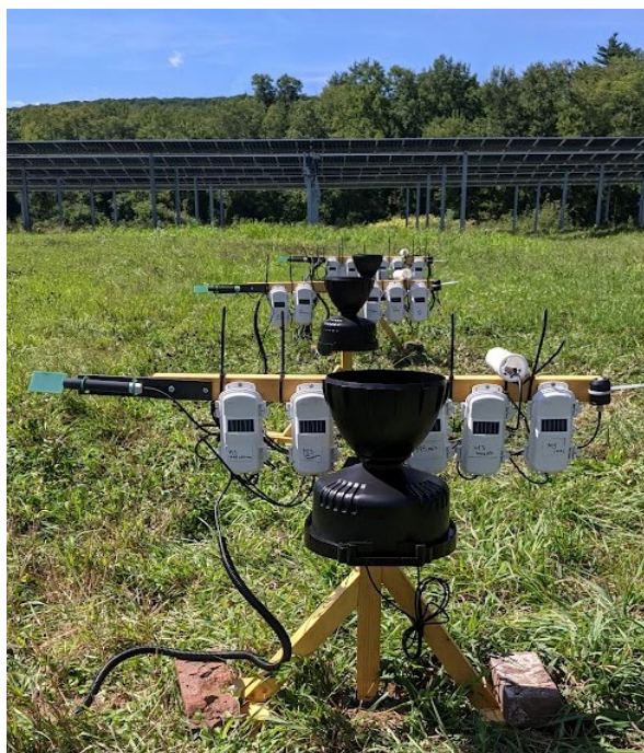
Figure 1: Sensors deployed in the field in a transect of three positions. Placing sensors in a transect allows for capture of unique “zones of influence” within the array, such as the different effect created by the dripline of the panel versus the reduced rainfall received underneath the impervious panel. The transect is also used in the control area of the study so that in-field variation is equally captured.
