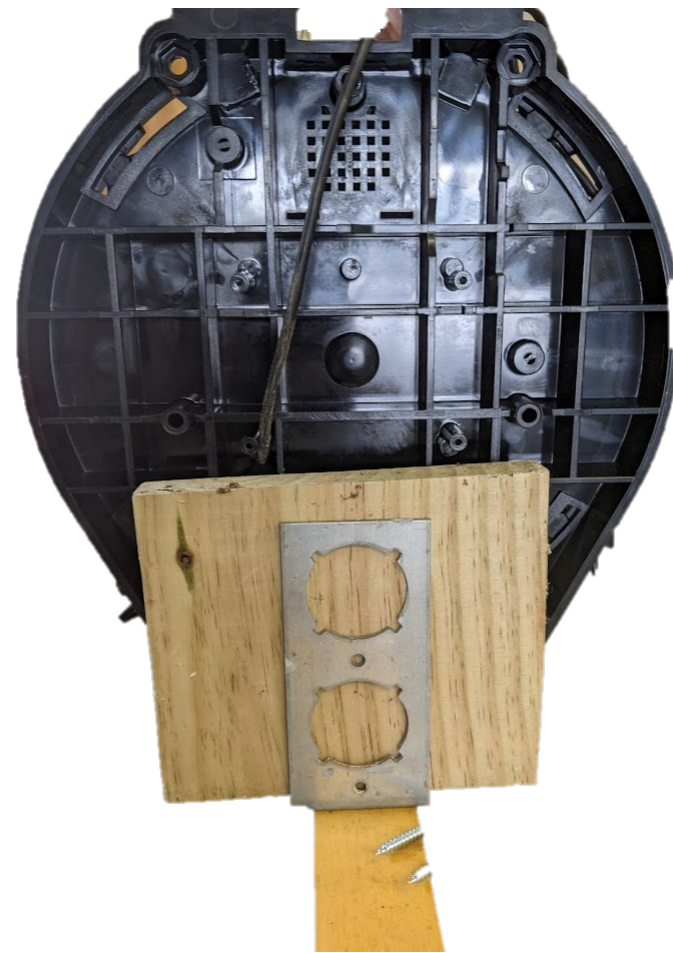
Figure 5. Bracket and shelf for the rain sensors. Note the wood shelf can and should be bolted to the bracket; bolt not pictured here. The wood should also receive waterproof finish.
