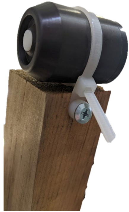
Figure 4. PAR sensor with the mounting cable connected to the back of the stand.
