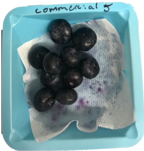
Figure 1. A sample of a drip loss assay of blueberries in a weight boat. The moisture has been transferred to the paper towel.
