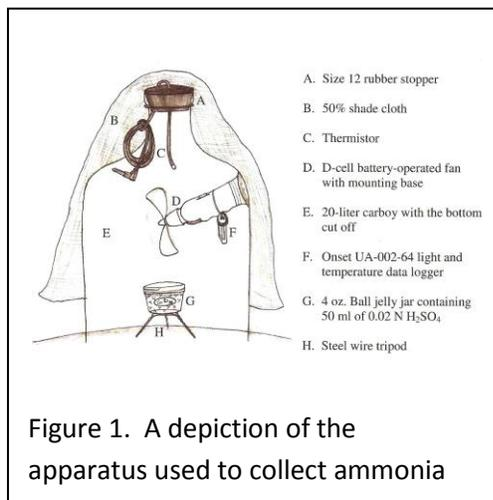
Figure 1. A depiction of the apparatus used to collect ammonia
