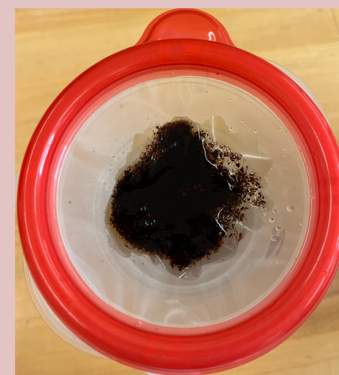
Figure 4: Sample contents in sieve, being sprayed with DI water to filter out particles <125 μm.
